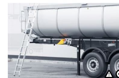
S Access ladder Thanks to its special shape, this access ladder enables risk-free entry and exit of the trough for maintenance and cleaning work.
