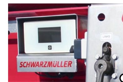
P Thermo trough temperature detection incl. 5 measurement points Sensors monitor the mixture temperature in the trough, thereby guaranteeing high paving quality. A recording device stores the data.
