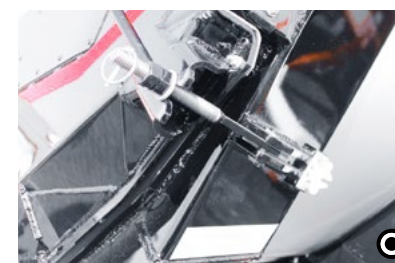
L Tensioning screws Viscous transport materials increase the pressure on the tailgate. In order to withstand this load, additional tensioning screws are fitted to secure the load.
