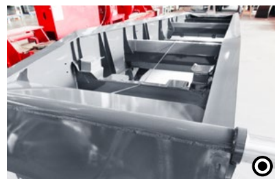
2 Torsion tubes Similar to the torsion box, these special cross-links ensure added tipper trailer stability throughout the tipping process.
