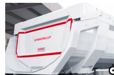
I Hydraulic tailgate The hydraulic tailgate can be opened fully hydraulically, meaning the whole opening is available immediately and even large stones can be unloaded without issue.
