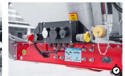
10 Brake and light connections The brake and light connections are clearly and compactly arranged at the front of the vehicle together with the electrical and hydraulic connections.
