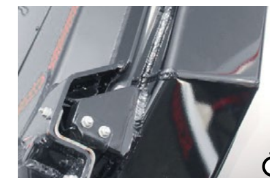
M Rubber seal Additional rubber seals in the tailgate area are a reliable means of ensuring that the necessary leak-tightness is guaranteed as far as possible.
