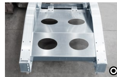
1 Torsion box A sophisticated, tried and tested solution for guaranteeing optimum stability in the tail area of the tipping trailer throughout the tipping process.
