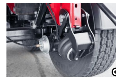
X Lifting axles Reduce tyre wear by means of automatic axle raising during empty runs, while serving simultaneously as a start-up aide.
