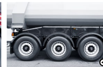
9 Single-wheel mud guards Schwarz Müller tipper trailers feature single-wheel mud guards. These protect other road users, and the trough, against stone chippings and dirt.
