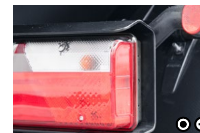
V Light protection In order to protect these from damage and coarse dirt as best possible, the tail lights are framed with their own sheet steel cover.
