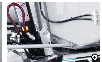
13 Central lubrication strip The 4 lubrication points of the tipper cylinder can be reached from a central lubrication strip, thus simplifying the lubrication process and saving time.
