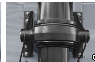
12 Four-point mounting The tipper cylinder is mounted at four positions (twice at the top and twice at the bottom). This creates unique tipping stability compared with a three-point mounting.
