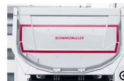
G Rear wall with tipping drain The rear wall is offset into the trough, causing the formation of a chute – the load's centre of gravity moves further forwards and increases the pressure on the tractor unit's rear axle.
