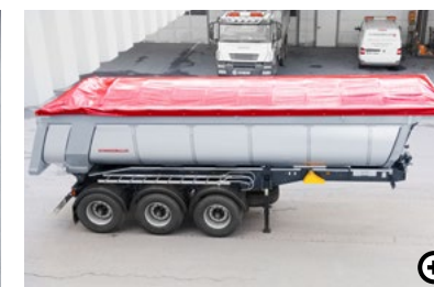
O Schwarz Müller cover Electric sliding cover with remote control for convenient opening and closing of the protective tarpaulin from the ground.
