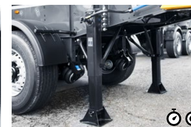
W Landing legs Schwarz Müller offers a choice of landing legs: either in the form of a steel or aluminium crank-handle leg or steel or aluminium support legs.
