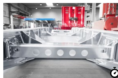
A Aluminium frame The optional aluminium frame brings an added weight advantage of 250 kilograms compared with the steel design.
