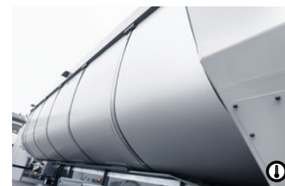
7 Thermo trough The trough is thermally insulated throughout. Asphalt mixtures can for example be transported to building sites at a higher temperature, contributing to a significant increase in paving quality.
