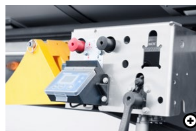
D Operating console Collective layout of control elements such as brake release valves, lifting and lowering device, trailer monitors or lowering lock for simpler operation.
