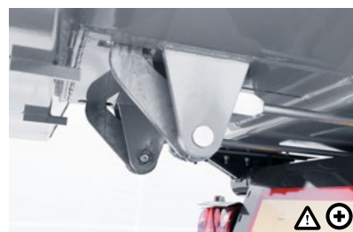
6 Automatic tailgate unlocking The tailgate is automatically unlocked by a special rod during the tipping process. This is also the mechanism which triggers automatic locking upon lowering.
