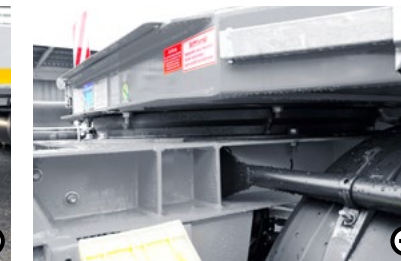
U Low-maintenance ball steering turntable The low-maintenance ball steering turntable reduces turntable lubrication frequency.
