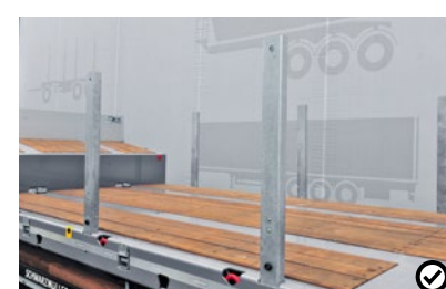
J Formed pipework Optional formed pipework can be accommodated in the designated pockets.
