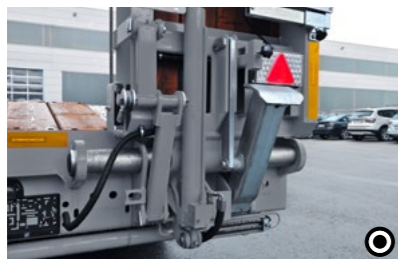
4 Folding supports on the ramps The folding supports extend automatically when the ramp opens. These prevent the trailer from shooting up at the front during the loading process.
