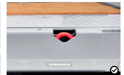
11 10 t lashing rings Fold-out lashing rings are intended for securing the goods for transportation.
