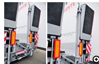
B Foldable two-piece drive-up ramp This is tipped downwards to allow driving onto the loading surface. The low angle of approach enables smooth loading of vehicles with reduced floor clearance.
