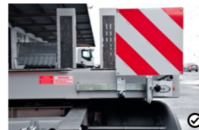
7 Pull-out warning signs These serve as a means of (variably) indicating vehicle width in order to guarantee the safe transportation of excess-width vehicles.
