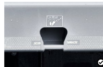
12 3 t lashing mushrooms The lashing mushrooms are intended, like the lashing rings, as a means of securing loads.
