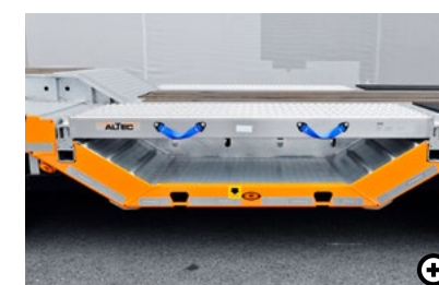
K Wheel recesses with covers Enable the transportation of high construction vehicles without exceeding the legal total vehicle height. Can be realigned using covers.
