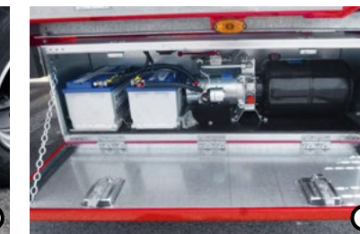
O Electrohydraulic pump assembly To avoid external hydraulic supply where the truck unit is not equipped with hydraulics.
