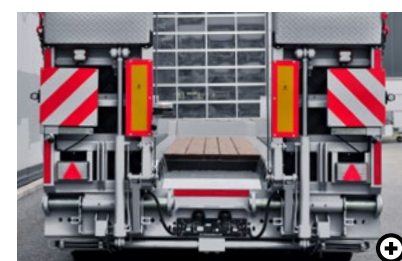
D Hydraulic sliding ramps Both ramps can be slid sideways hydraulically.
