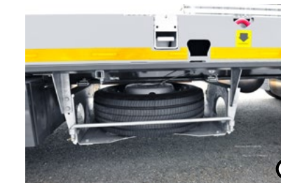
T Spare wheel holder This is an easy way to transport a replacement wheel en-route.
