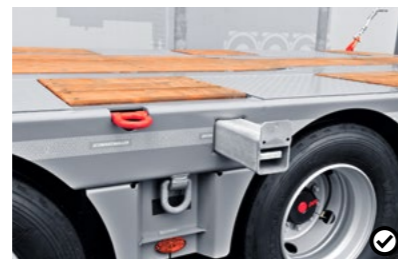
5 Pull-out extensions The load carriers can be extended up to a width of three metres, enabling the transportation of wider vehicles.
