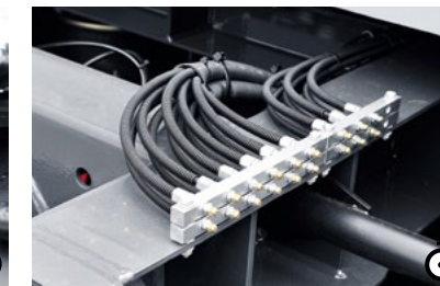
V Central lubrication strip From here the lubricating points of the ball-cage assembly and the axles can be reached, thus simplifying the lubrication process and saving time.
