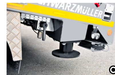
E Hydraulic support feet at the end of the vehicle Hydraulic support feet at the end of the vehicle provide added stability while loading. These prevent the trailer from shooting up at the front.
