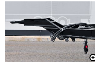
C1 Offset drawbar The offset drawbar serves as a means of levelling the coupling height of the truck and the trailer.
