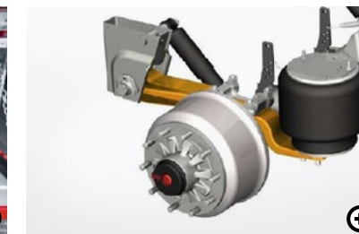
P Air suspension Air bellows are used for the trailer suspension.
