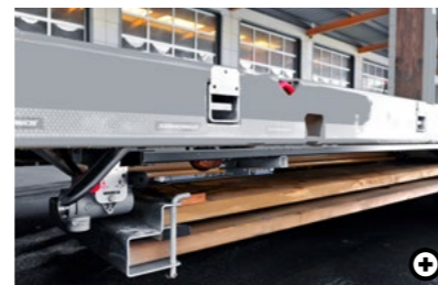
6 Storage compartment for widening boards The wooden planks for extending the loading surface are located in a storage compartment underneath the loading surface.
