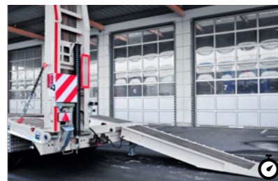
2 Foldable single-piece drive-up ramp The foldable single-piece drive-up ramp folds downwards to allow driving onto the loading surface.
