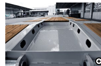
F Excavator trough The excavator trough is a recess in the ramp slope for accommodating an excavator arm.
