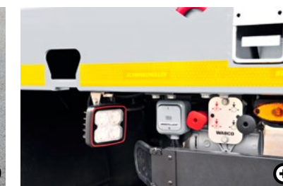
S Work lights The work lights provide extra lighting during the loading and unloading process.
