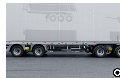
A Straight platform The straight platform version features a horizontal loading surface.
