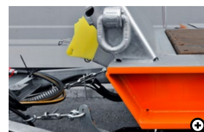
M Cylinder stem Prevents a loaded cylinder from slipping forwards.
