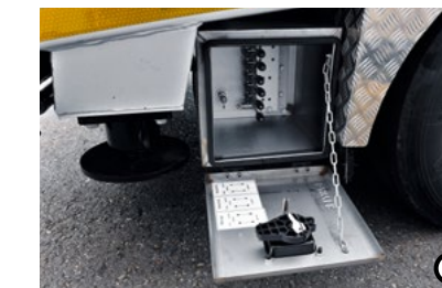
N Stainless-steel box for ramp control This control unit serves to raise and lower the drive-up ramp. Optionally available for the sideways sliding of the ramp too.
