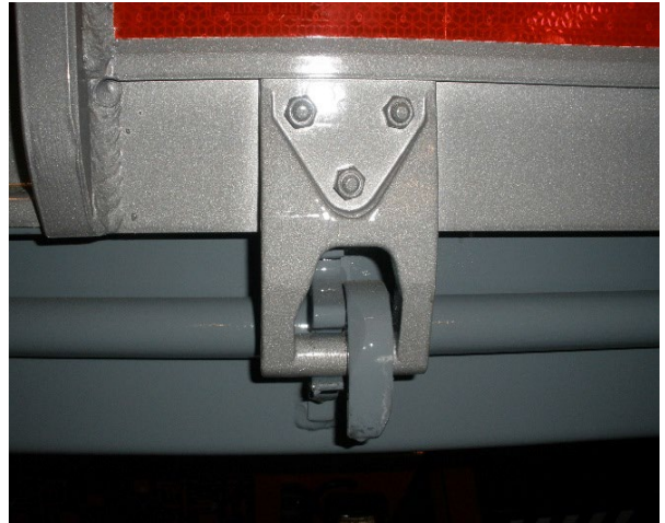
Hinges: Check the weld seams for cracks, check that the screws are tight
