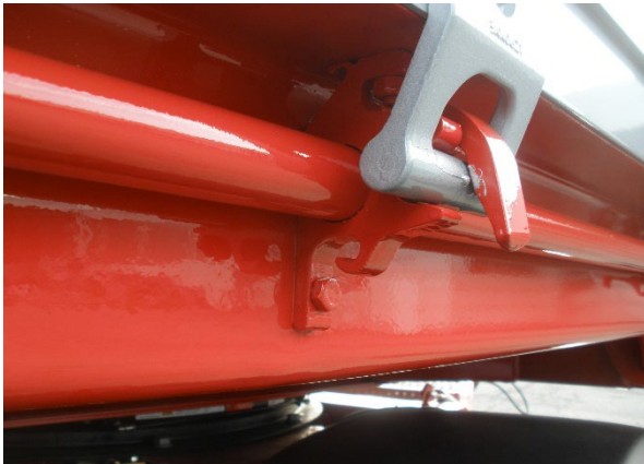
Central latch: Visual inspection for wear, play, screw fitting etc.
