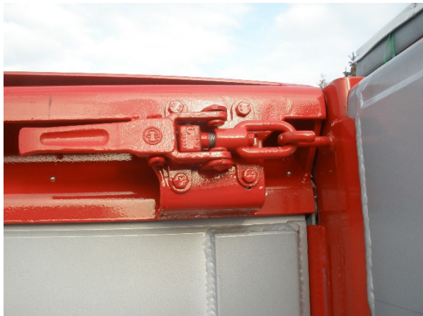
Latch at top rear wall crosspiece: Check for tightness and operability
