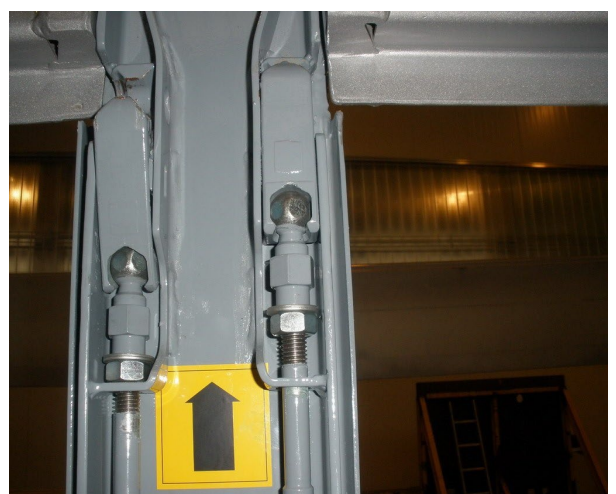
Front wall, central post(s) and rear corner posts: Check operability of latch
