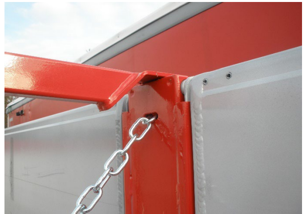
Central stanchion link or chain connection: General visual inspection
