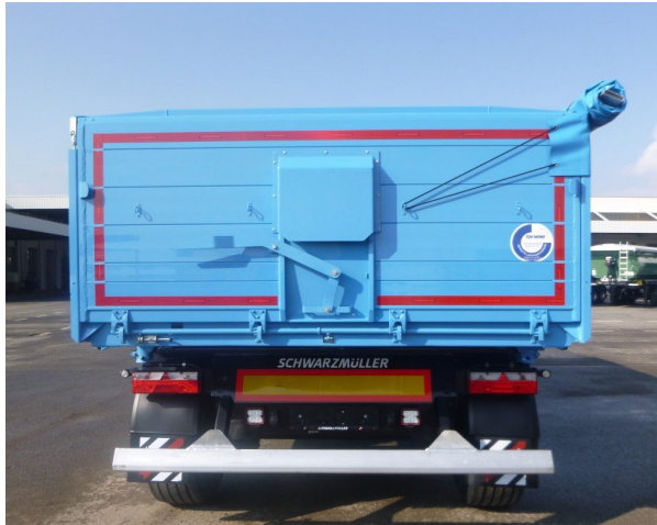
Rear wall: Check the weld seams for cracks
