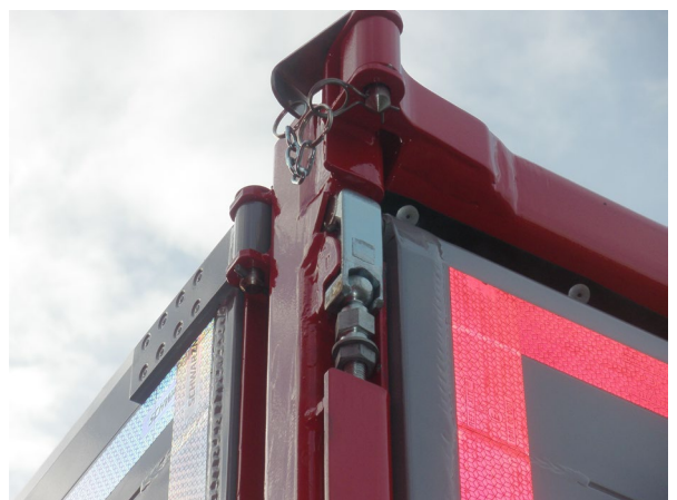
Check all moving attachments (hinges, latches, bolts, pins etc.) for wear and operability
