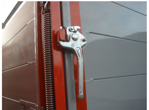
Latch: Check for wear and operability
