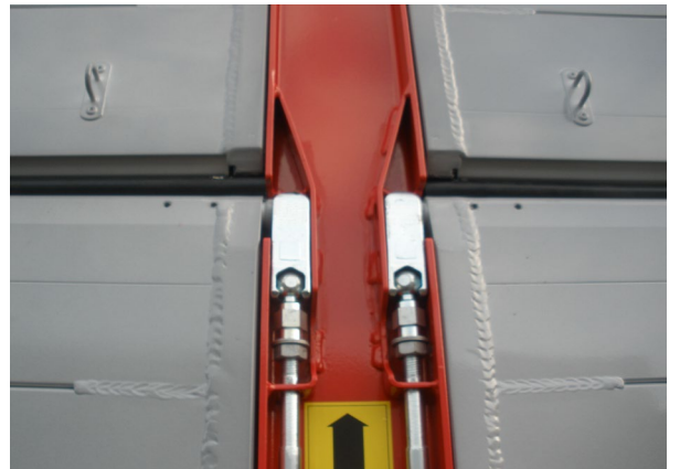
Inner and outer side panels: Check the weld seams for cracks
