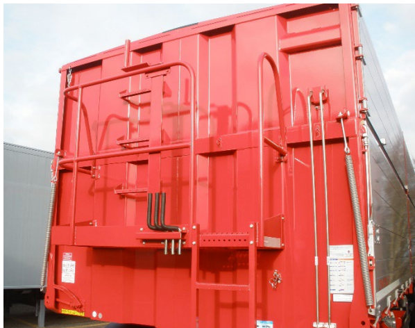
Check all weld seams for cracks, Latches, hinges etc.: General visual inspection
