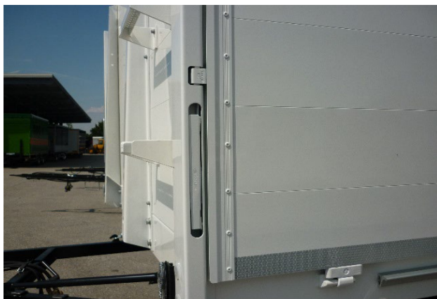
Check that the screw fitting of the front corner column is tight
