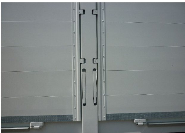
Central and corner posts (front and rear): Check operability of latch
