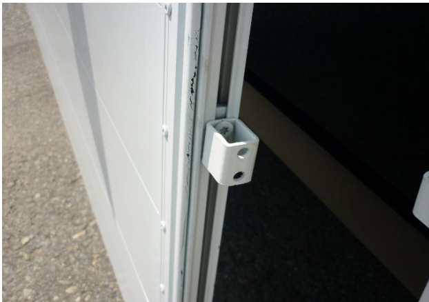
Check that the holding hooks are tight and undamaged
