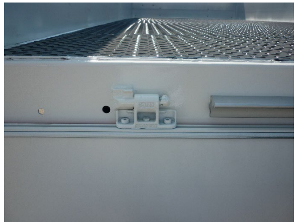
Check the hinges for operability and damage. Conical hinge: Check the weld seams for cracks
