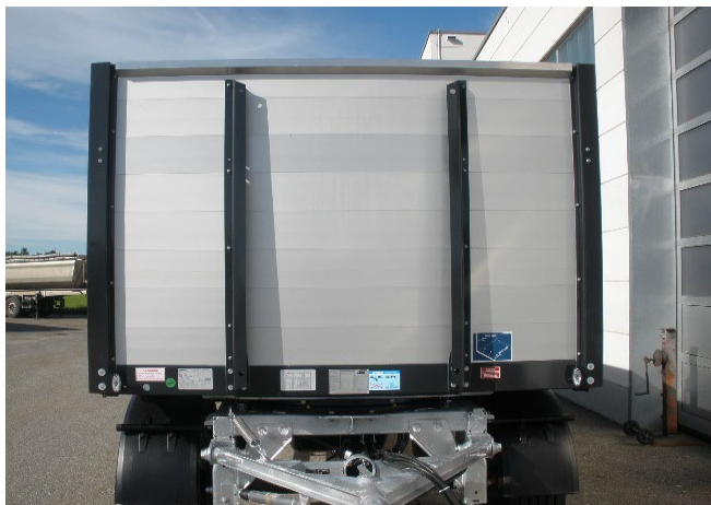
Check that all rivets and screws are tight
