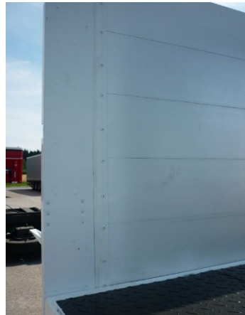
Side panels: Check that the rivets are tight
