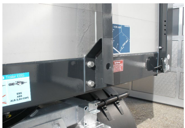
Check that the screw fitting of the front wall support is tight
