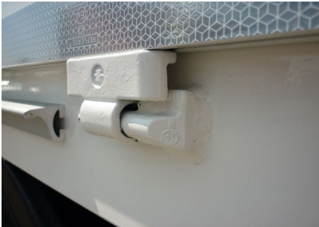
Check the hinges for operability and damage. Conical hinge: Check the weld seams for cracks
