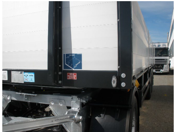
Tool holder: Check that all rivets and screws are tight
