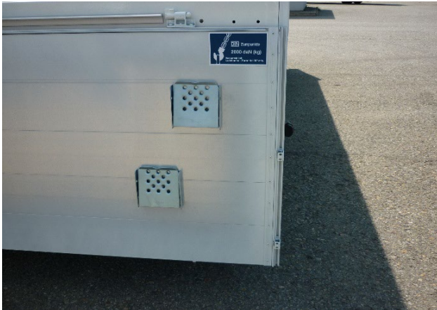
Rear wall: Check that the rivets are tight
