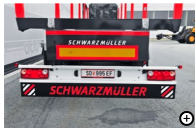
3 Aluminium underride guard This ensures that the trailer or semi-trailer cannot be underridden, improving safety for other road users. Also available in steel or stainless steel.
