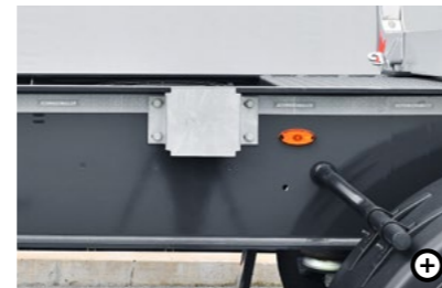
2 Clamshell protection plates Clamshell protection plates on the side members prevent the clamshell from causing damage during unloading.
