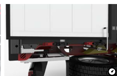
17 Rear door holding fixtures Hold back the opened rear doors to prevent them from closing inadvertently.
