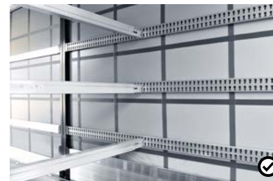
L2 Steel slot-in slats with attachable blocking slats Instead of V-type slats, steel slot-in slats with a special hole pattern are installed for securing the cargo at the rear end.
