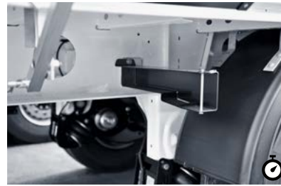
H Slat retainer The retainer provides a safe and convenient storeroom for unneeded side slats.
