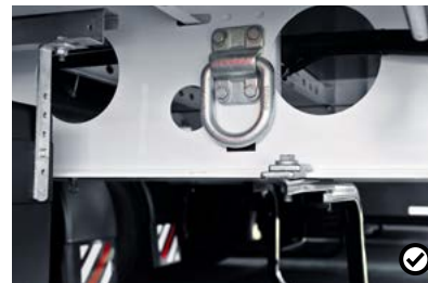
K Blocker tie rings Semitrailer securing elements required when using a ferry.
