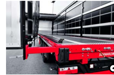
T Portal frame with crank Crank out the rear corner posts to generate more loading width at the rear end.
