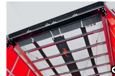
V Inflatable Air-Pipe restraints Inflatable roof-mounted restraints create an inclination down which rain water can run off before freezing and building up ice that may put other road users at risk.
