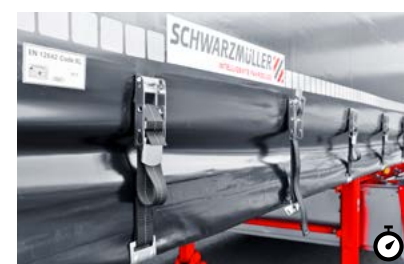
2 Over-centre tarpaulin tensioners The special-purpose tensioners attach the tarpaulin to the outer frame while supporting the tie-down of the cargo.
