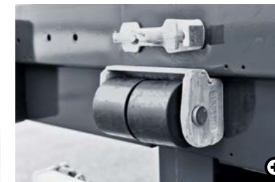
Y Butt roll Moving fenders are used when backing up to loading ramps. The rolls avoid damage caused by up and down movements while loading.
