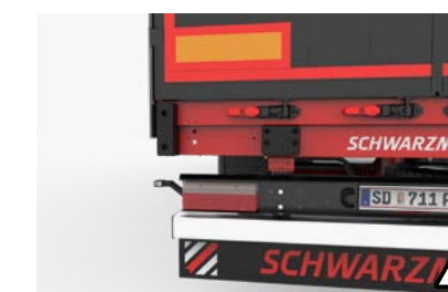
18 Fenders These rubber fenders protect the vehicle body against damage when backing up to loading ramps.
