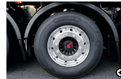
W Aluminium rims The lightweight rims reduce the vehicle's tare weight by another 120 kg.
