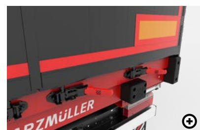
6 One-hand door latch One hand is enough to operate the rear door latches.
