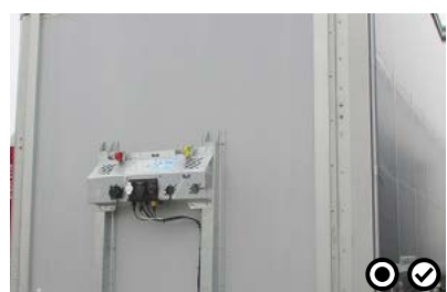
11 Front wall The front wall saves an extra 60 kg of weight and its tremendous robustness requires no separate protection of the inner front wall side.
