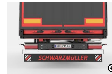
X Rubber delta May serve as fender when backing up to loading ramps.
