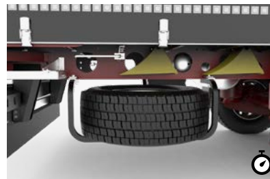
N Spare wheel bracket Safe and convenient means of transporting a spare wheel.
