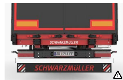
14 Underride protection Prevents other vehicles from underiding the rear trailer end in conformity with new EU regulations coming into force in 2021 (higher test loads).
