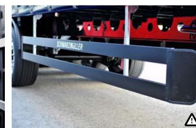
13 Side impact protection Statutory cyclist protection to prevent persons from falling down in front of the wheels.
