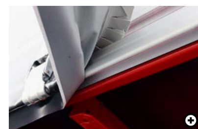
1 Tarpaulin hooking rack Vertically attaches the side tarpaulin to the outer frame. Ensures a perfect connection without the tensioners standing askant.
