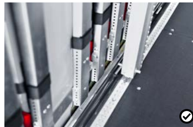
L1 Set in rails for blocking poles Mounting rails set into the floor and roof are used to install the upright blocking poles. The poles secure the cargo at the rear end.
