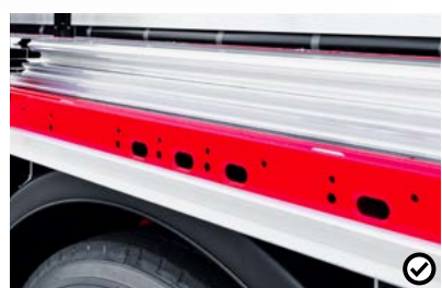
8 Perforated external frame The perforated external frame not only allows for the lashing points but also for hooks for securing the cargo at any point.
