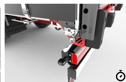
20 Ratchet tensioner For quickly tensioning the side tarpaulins. Mounted on the left and right rear ends.
