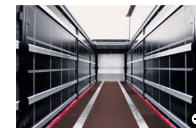
12 Force-controlled resin-coated floor 28 mm thick to support stacker axle loads up to 7,200 kg. Paper models have a double floor (28 mm + 12 mm, stacker axle load: up to 8,000 kg).
