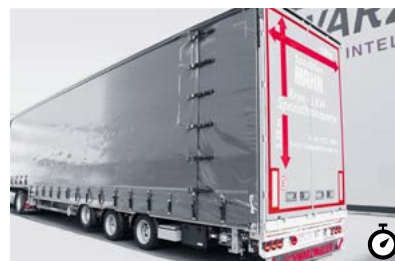
Q Folding tarpauling for excess width Tarpauling with integrated extra material lengths. If not in use, the excess tarpaulin material attaches to the inside by means of a Velcro strip.
