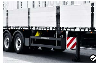
M Side panels Semitrailers can be equipped with side panels.
