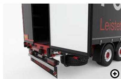
7 Welded rear door profiles The aluminium profiles of the rear doors are installed vertically and welded up to one another. This prevents the profiles from slipping or becoming loose in the course of time.
