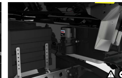
F Central lubrication unit
